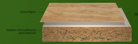
When compared directly to blended Fir particleboard, Pine substrates offer critical manfacturing advantages:
